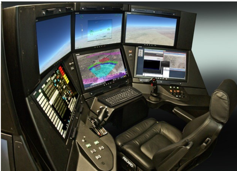
Fig 5. Advanced Cockpit Ground Control Station. General Atomics Aeronautical Systems, Inc. 2015.
