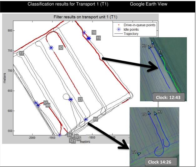
Figure 8 - (Right side) Trajectory of Transport unit 1 (T1) is plotted, along with idle points in blue colors and driving-in-queue points in red color. Numbers in squares are duration of the idle period in seconds. (Left side) Two parts of the trajectory of T1 is viewed in Google Earth along with the trajectory of the other vehicles. The thick part of drawn trajectories corresponds to 60 seconds.
