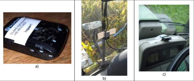
Figure 2 – a) Close-up photo of the GPS receiver and of the receiver taped to the window of a forage harvester and on the dash board of a tractor.
