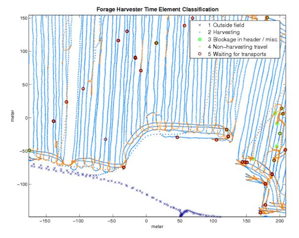
Figure 11 - Harvester classification results. The harvester initially harvests the boundary of the field to make room for the transport units and the later u-turns. Because of this the harvester will not harvest any material in the u-turns. In the figure it can be seen that the classifier successfully classifies points on the u-turns at the boundary of the field as "Non-harvesting travel".
