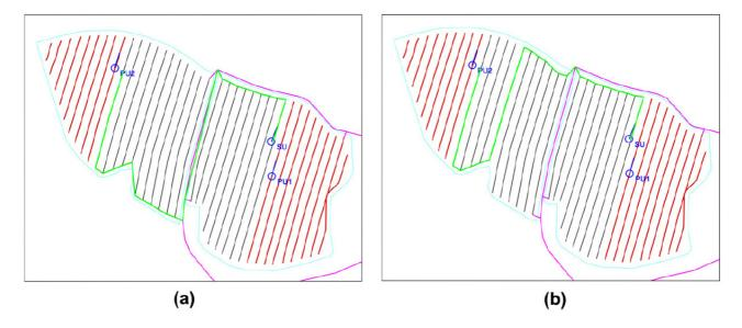
Figure 1 - The location of the SU (transport unit) and PU (harvester) are the same but optimality criterion is in a) time and b) distance, which gives two different paths.
