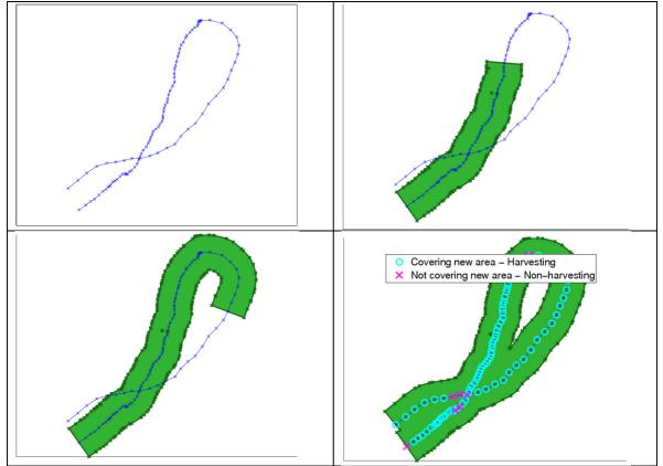
Figure 5 - From upper left to lower right, the plots show how the worked polygon is built iteratively from the trajectory (upper left plot). The points where new area is covered are classified as "Harvesting" otherwise "Non-harvesting".
