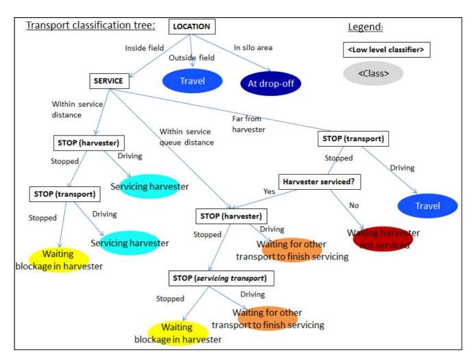
Figure 10 - The TRANSPORT classifier is described by requirements to the results of the lower level classifiers LOCATION, STOP and SERVICE.
