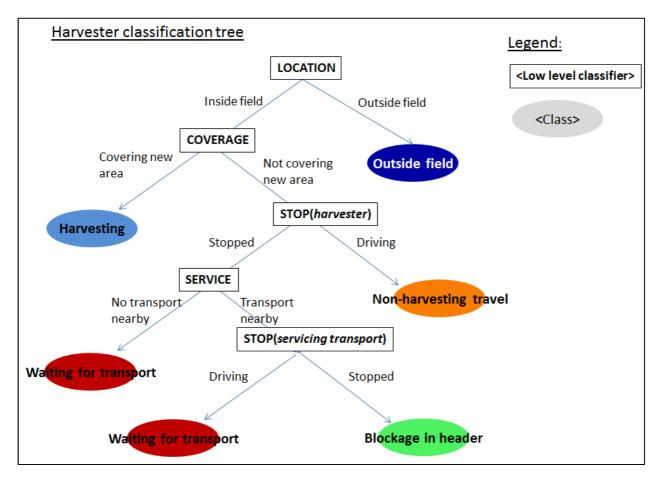
Figure 9 - The HARVESTER classifier is described by requirements to the results of the lower level classifiers LOCATION, COVERAGE, STOP and SERVICE.
