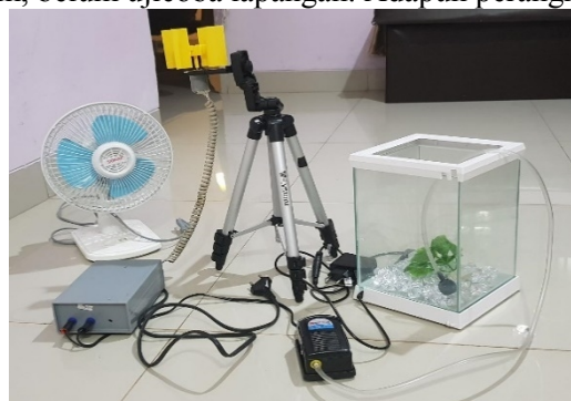
Gambar 2. Prototipe Aerator Kincir Angin
