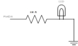
Gambar 5. Rangkaian indikator lampu LED
