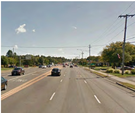
Figure 22. Genesee Street in DeWitt, NY. This is an example of a typical commercial street in a sprawl setting. Streets such as this have numerous wide lanes with no bike lanes making bicycle travel dangerous if not impossible. Sidewalks are located very near to vehicular drive lanes creating an uncomfortable experience for pedestrians (Image credit: Google Maps).
