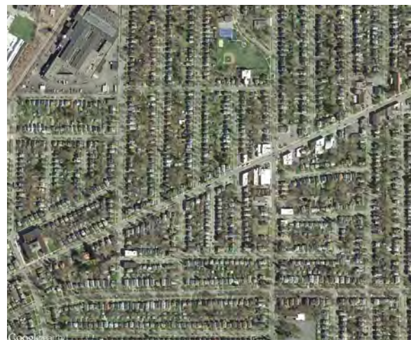
Figure 21. The street network in the 19th Ward, Rochester, NY. This is a typical street pattern found in a traditional residential neighborhood. Local residential streets have a great deal of connectivity to arterial, collector and other local roads because of the gridded street pattern. This pattern significantly reduces traffic (Image credit: Google Earth).
