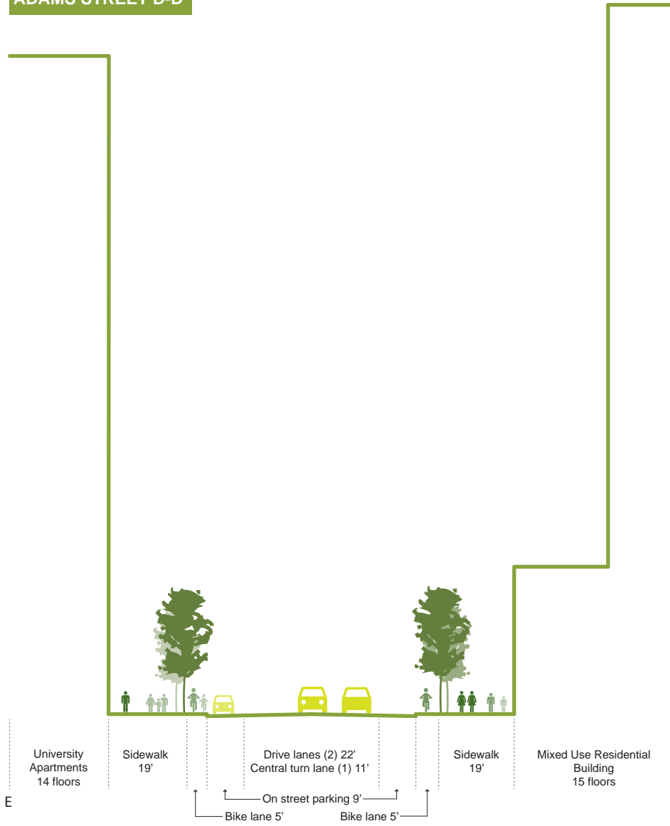
Figure 57. Adams Street, section D-D': This section displays Adams St. just to the west of Almond Blvd. Adams St. contains four drive lanes, wide sidewalks, bicycle paths and parking. Adams St. has been converted from one way to two way traffic and will serve as a crucial east-west connection between the Downtown and University Hill neighborhoods. Adams St. will feel less enclosed than other Downtown East streets due to the street's extra lanes and the lower heights of the PTSD building and buildings within the Pioneer Homes development.
