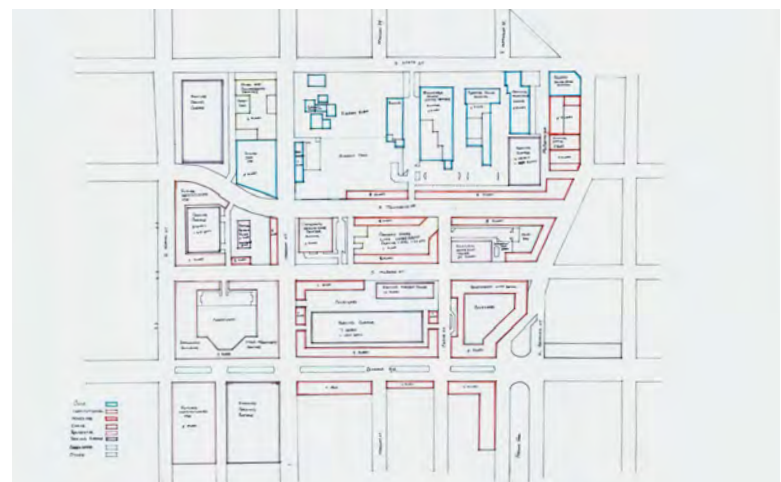
Figure 31. A further iteration of Downtown East created with pen and marker on trace paper that continues to study the street network. In this iteration all medians have been removed except for those on Almond Blvd. and a short extension of Forman Park across Almond Blvd. This created larger parcels and allowed them to more easily meet parking requirements. For instance, in this iteration the Madison St. extension has been replaced by a large centralized parking facility. Additionally, the northern curve of Townsend St. has been straightened to accommodate a parking facility to the west. Liner buildings continued to mask undesirable views of parking facilities and service entrances. The Upstate University Health Care Center at 90 Presidential Plaza was still included in this iteration. Ultimately, its location was used for the Central Plaza.
