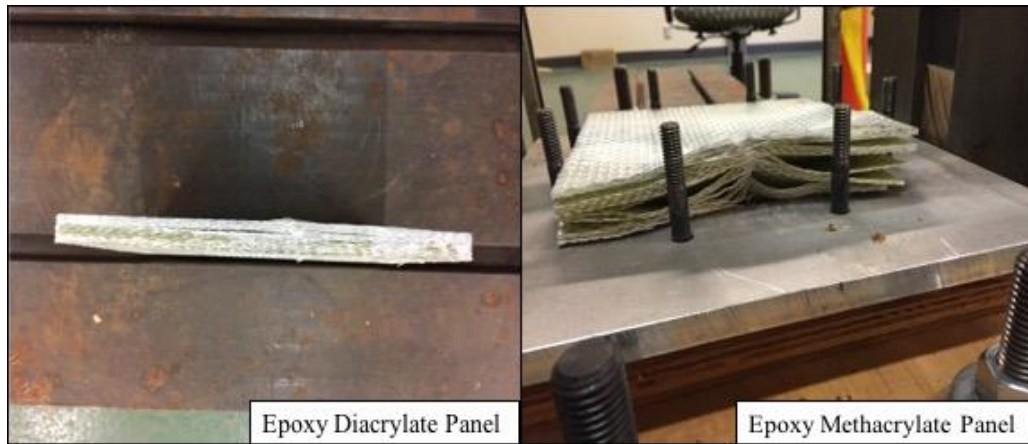
Figure 7. Epoxy Diacrylate panel and Epoxy Methacrylate Panel Showing Different Delamination after Impact Test (600 ft lb) When Cure Time was 15 + 15 Minutes
