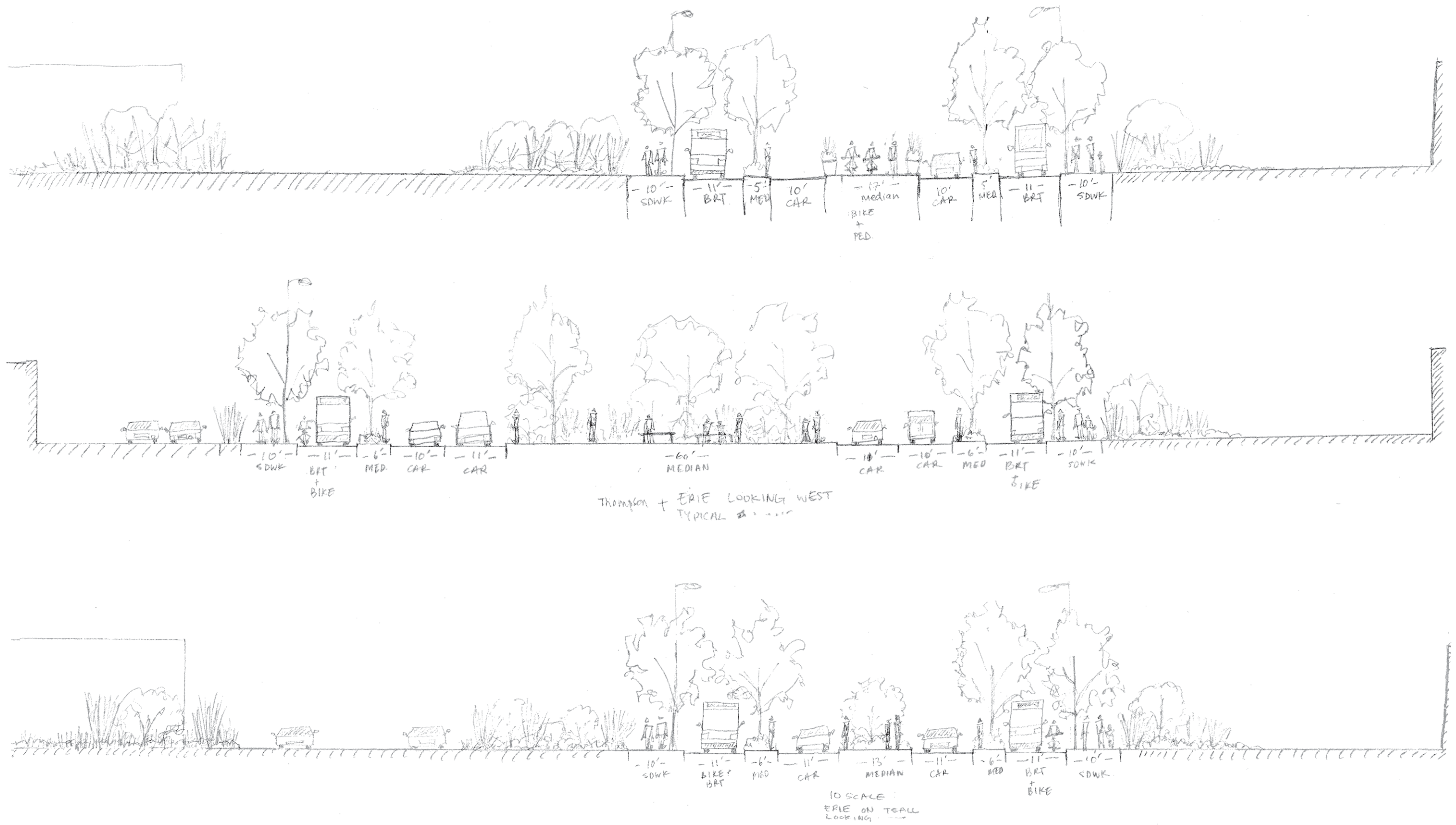
Figure 16C: Iterative Designs - Location options for BRT lanes, bike lanes, vehicles lanes, sidewalks, medians and shared and non-shared lanes
