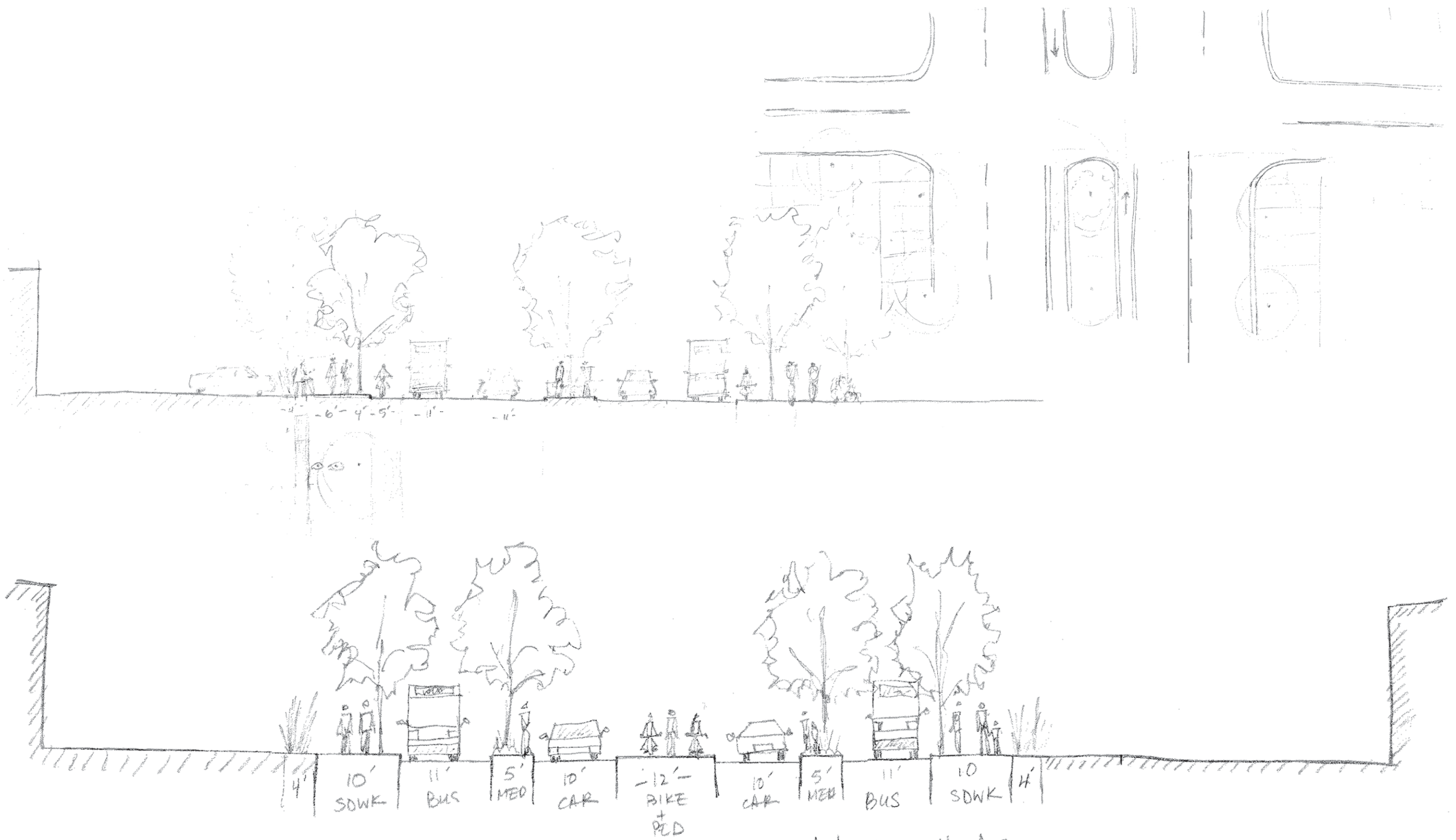
Figure 16B: Iterative Designs - Location options for BRT lanes, bike lanes, vehicles lanes, sidewalks, medians and shared and non-shared lanes
