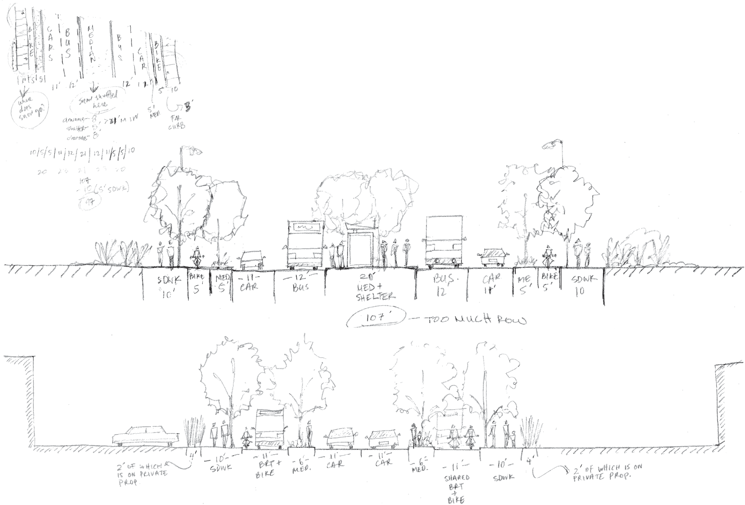
Figure 18A: Iterative Designs - Location options for BRT lanes, bike lanes, vehicles lanes, sidewalks, medians and shared and non-shared lanes
