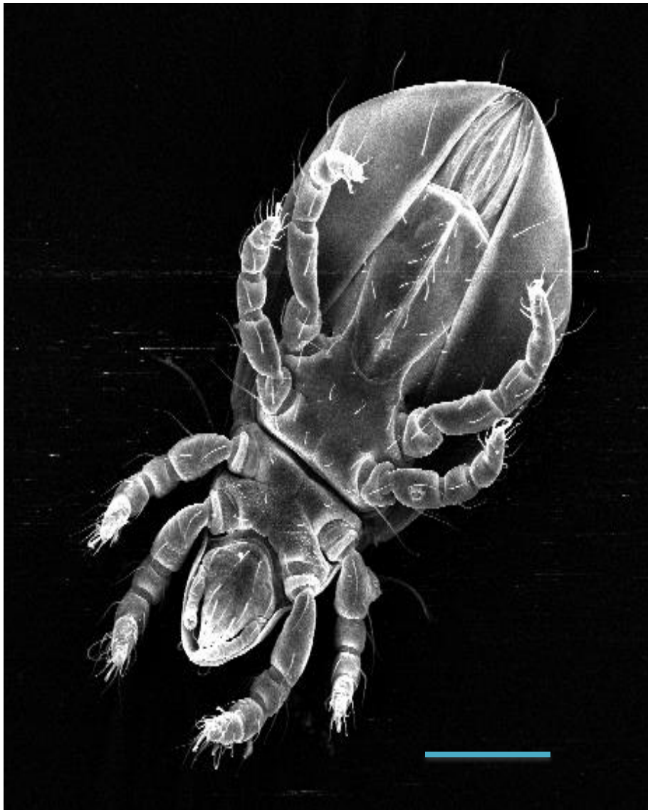
Figure 4a/b: SEI of a mite body. Image was taken at a working distance of 11mm and an aperture of 1. These images show amazing contrast and surface detail of the mite. Each structure is extremely distinct and clear. The background is very dark, especially on the left, meaning there is very little charging. SS 10, AV 20.0 kV, Mag (left) 200x Mag (Right) 500x Bar= 20nm
