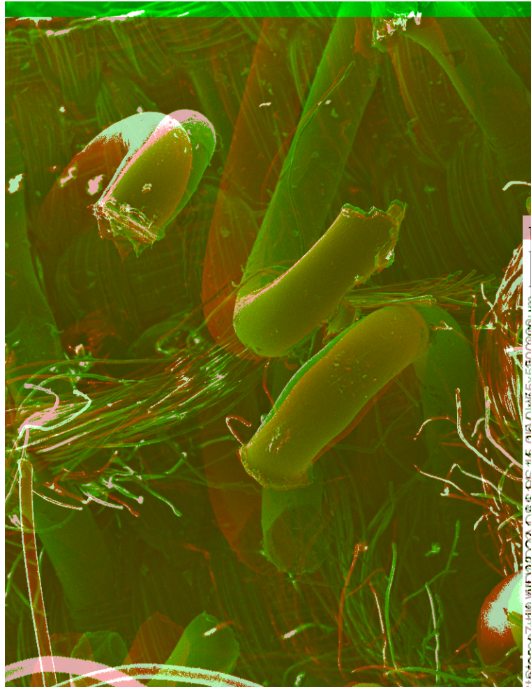
Figure 6. Stereo Imaging: Red/green stereo image of two SEM images of Velcro, combined using Adobe Photoshop. SEM images were captured at a spot size of 14 chevrons, 55X magnification, 23 mm working distance, objective aperture of 1, accelerating voltage of 15 kV, and tilts of +7 and +19 degrees. Image size is 4x5, 200 pixels/inch.
