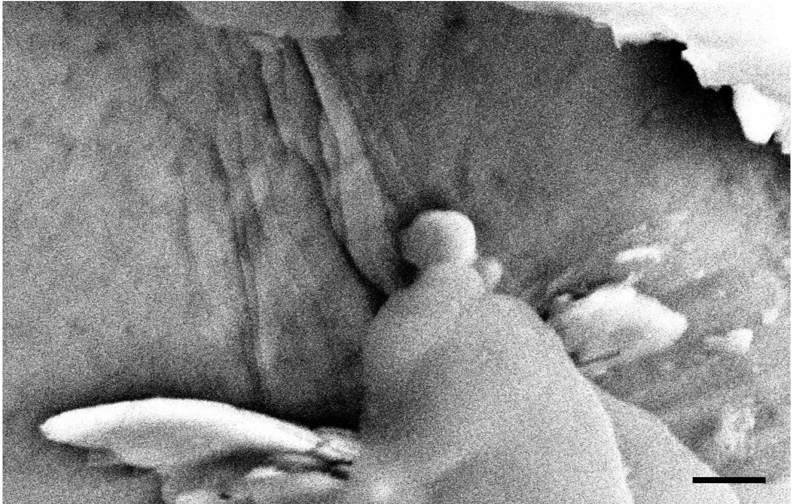
Figure 2. Hardest Image to Capture: Secondary Electron Image of a watch gear's residue captured at a spot size of 10 chevrons, 6000X magnification, 21 mm working distance, objective aperture of 1, and an accelerating voltage of 25 kV. Micron bar= 2 \mu m
