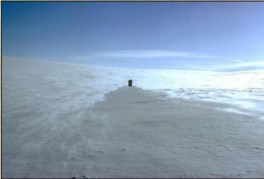
Snow shadow created by 1.2m wide cylindrical shed (Tabler 2003)
