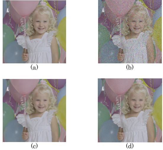
Fig. 14 Simulation results. (a) Original (noise-free) image. (b) Corrupted image with 10% noise. (c) Median filter. (d) Proposed filter.
