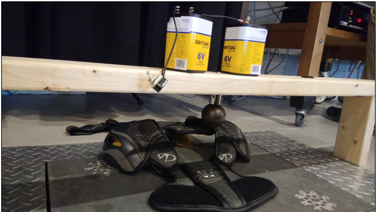
Figure 3. Drop Mechanism with Shoulder Pad
