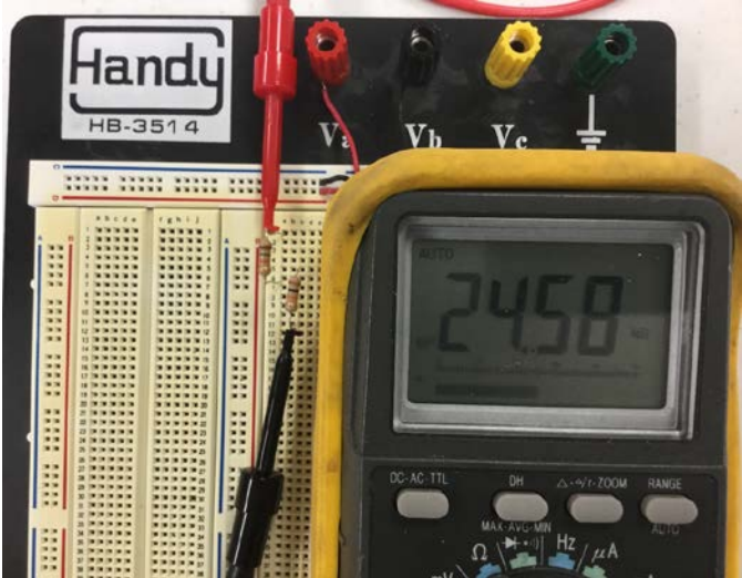
Figure 4: Physical breadboard setup for resistors in series
