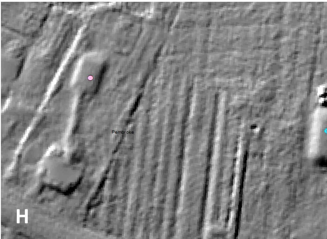
FIGURE 4 (continued) Views of septic leachfields in Oblique imagery. G) Failed Septic system that appears to be short circuiting. H) Hillshade from LIDAR derived topography showing a raised septic system connected to a house.
