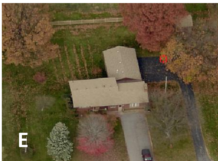
FIGURE 4 Views of septic leachfields in Oblique imagery. A) Example where individual leachlines are darker than surrounding areas. B) Example where the leachfield appears darker than surrounding grass. C) and D) same leachfield taken in March, and April. Note the difference in shading after the growing season kicks in. E) and F) leaves accumulating in microrelief associated with leach field.
