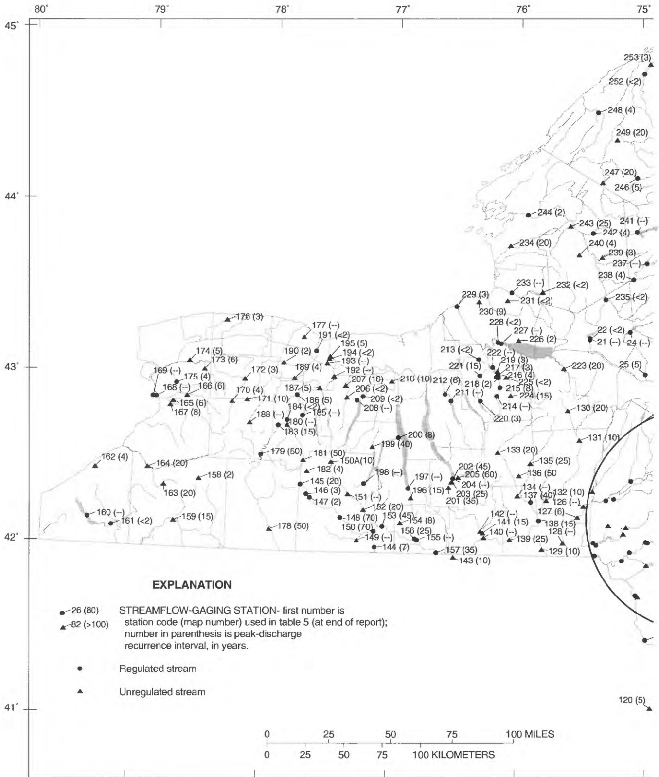
Figure 10. Locations of streamflow gaging stations and peak discharge recurrence intervals for the floods of January 19-20, 1996 in New York. (Data given in table 5 at the end of the report).
