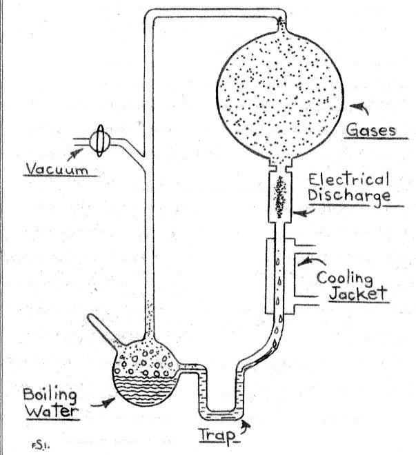
Miller made amino acids by circulating methane (CH<sub>4</sub>), ammonia (NH3), water vapor (H20) and hydrogen (H2) past an electrical discharge. The amino acids collected at the bottom of the apparatus and were detected by paper chromotography.
