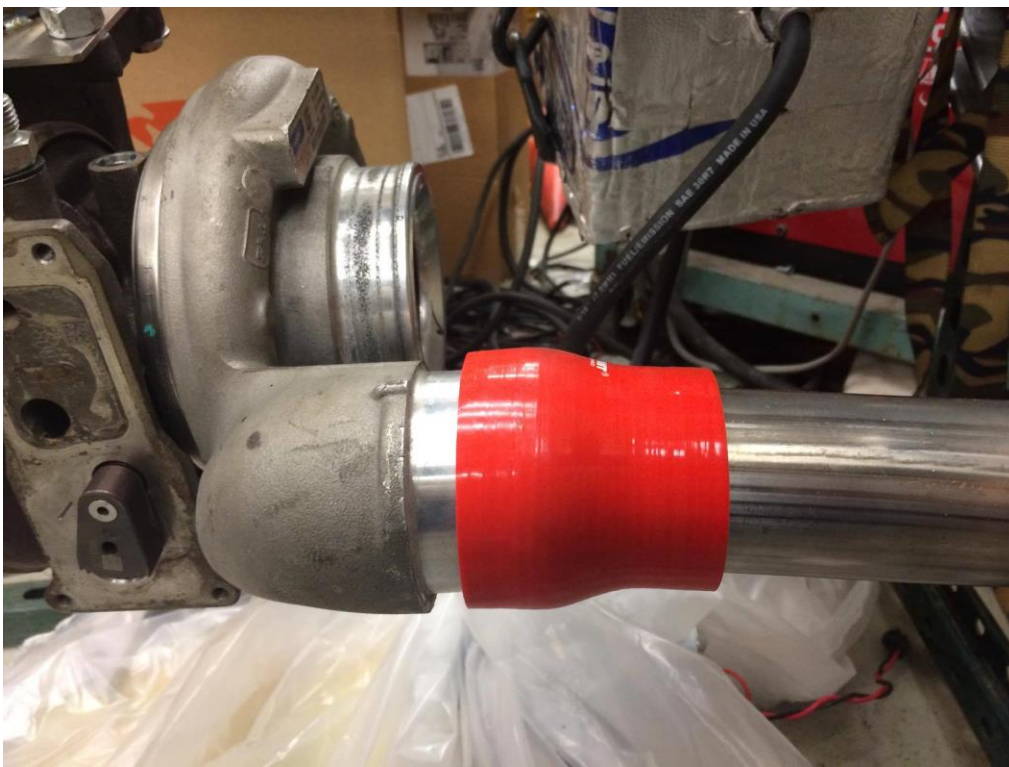
Figure 11: Connection between Turbocharger and Combustion Chamber Inlet
