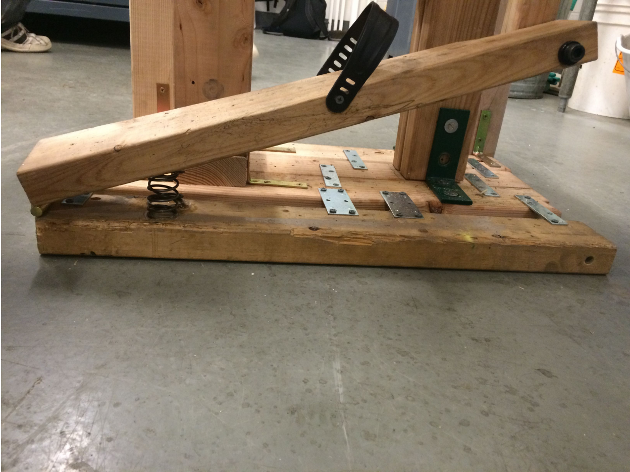
Figure 34: Pedal with springs and strap
