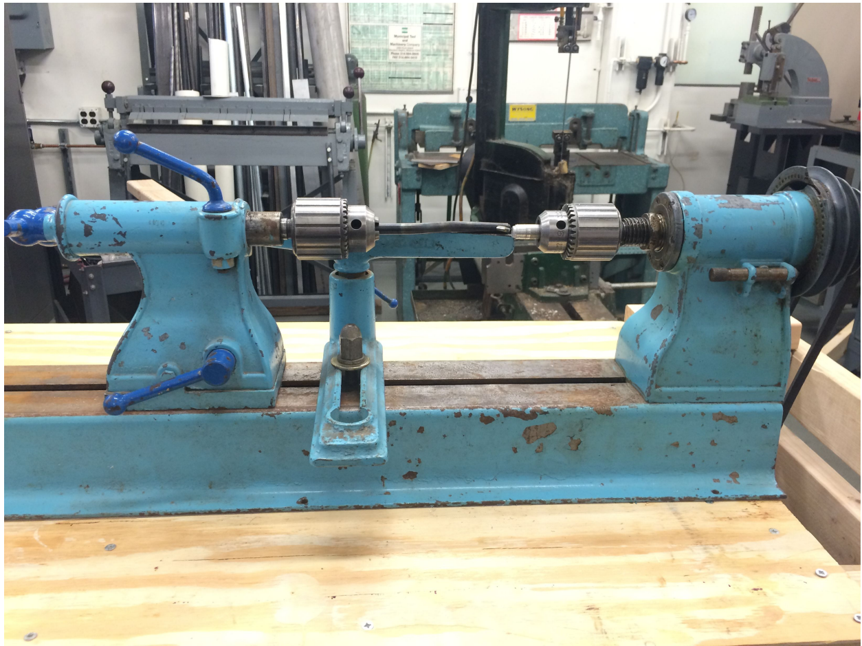
Figure 31: Lathe and custom cutting tool
