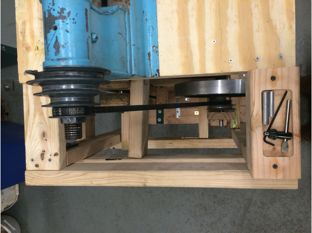
Figure 22: Top-down view of lathe to flywheel connection
