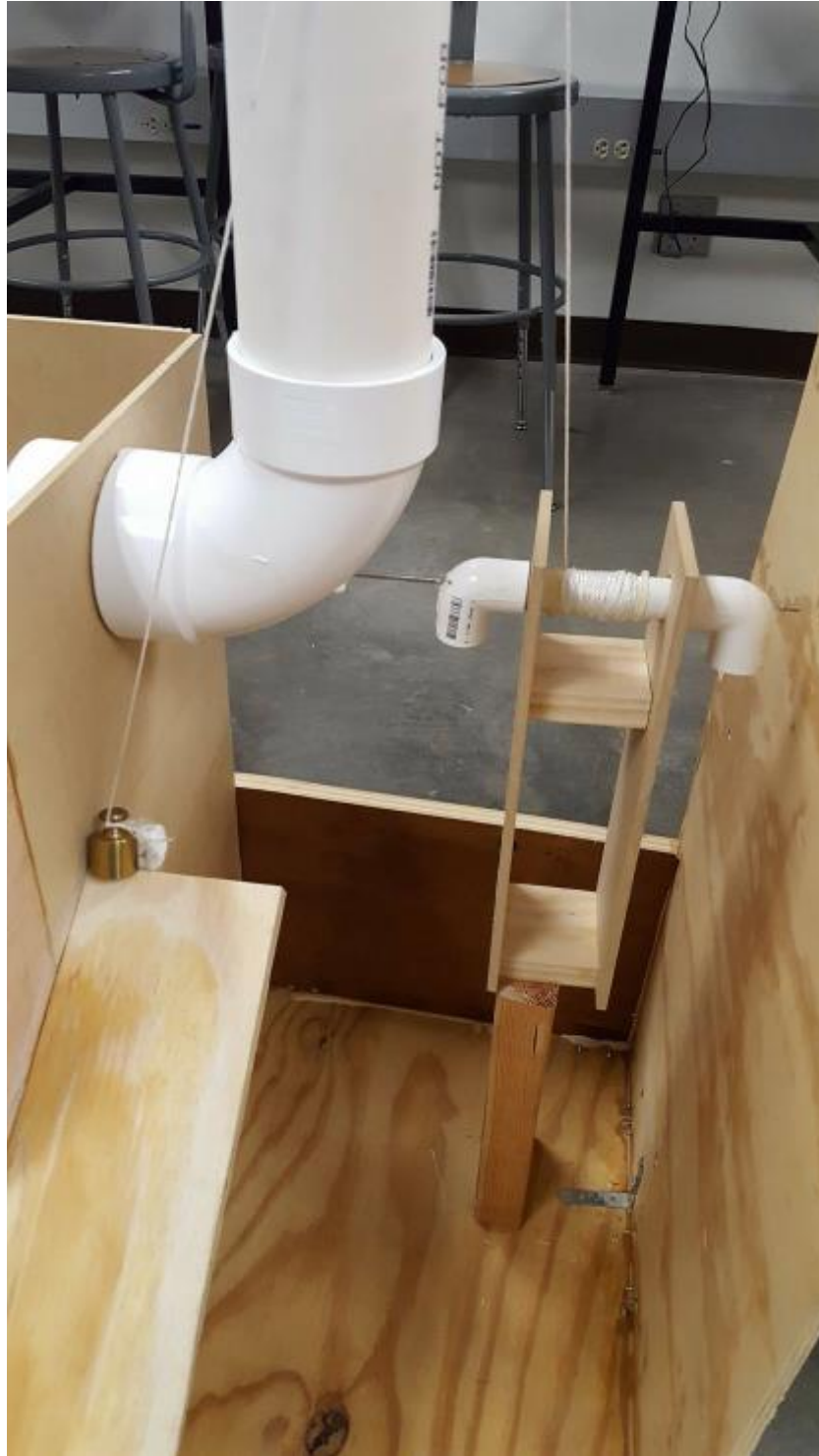
Figure 28: Picture of fan rotational mechanism attached to a pulley and weight.
