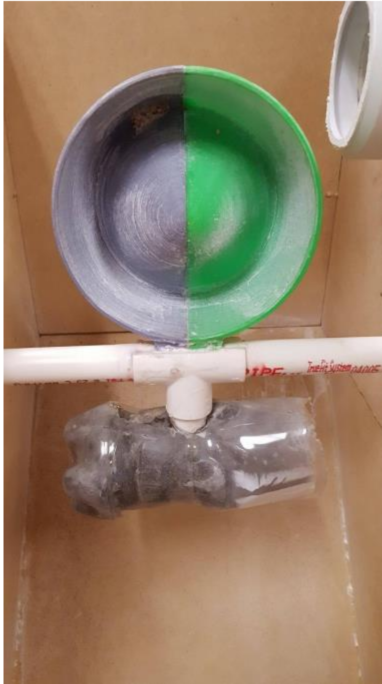
Figure 26: Picture of the seal with the counterweight that holds the waste.
