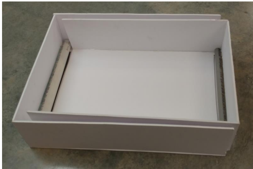
Figure 7: Underside of Prototype Revealing Sliding Mechanism
