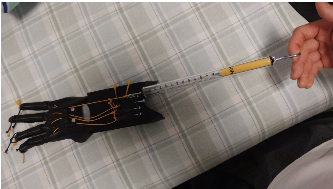
Fig. 33: A spring dynamometer was used to test the tension force.
