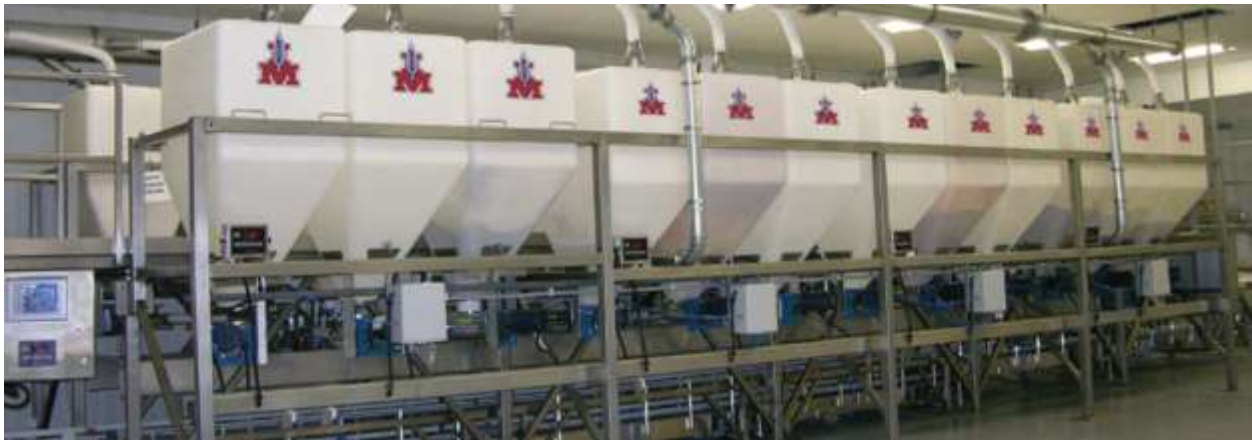
Figure 1: Ingredient Masters’s Large-scale dry ingredient dispensers (material specific)
