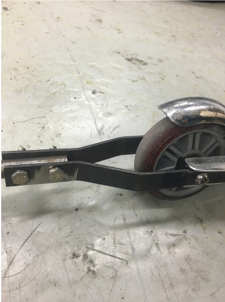
Fig. 22: Machined flanges attaching to the outer section of the wheel.
