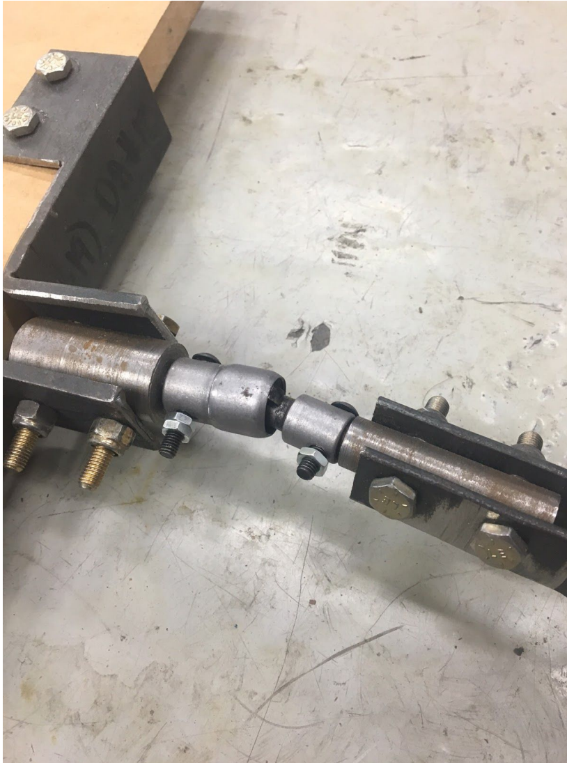
Fig. 22: View of ball and socket joint part attaching the trailer to the flange.
