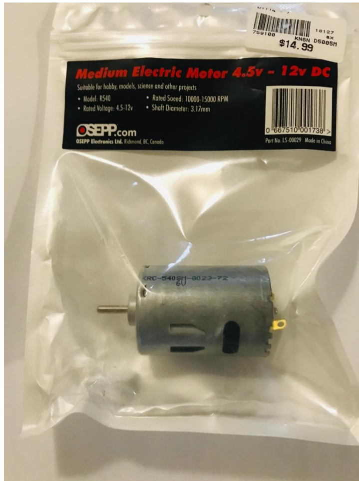
Figure 18: DC motor that will be used to turn the lead screw
