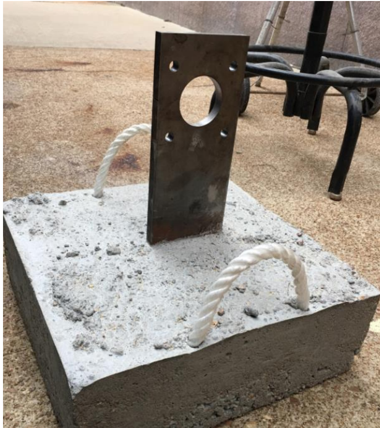
Figure 26 – Rear support set in concrete to fix the rear hubs of the chassis
