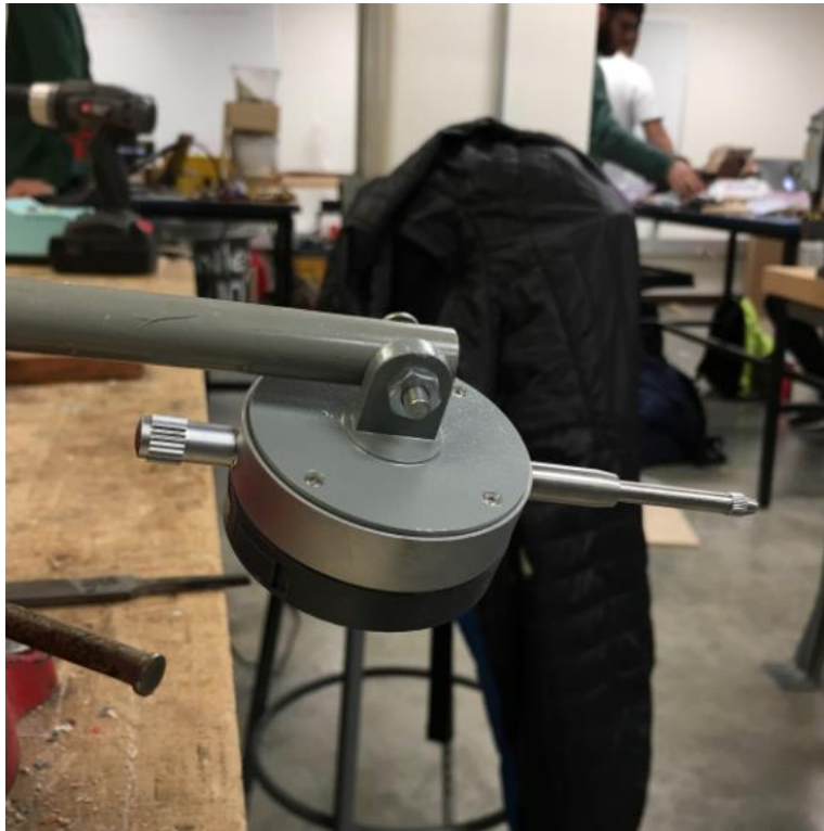
Figure 25 – Dial indicator with extension rod attached
