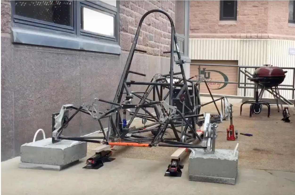
Figure 29 – Fully assembled torsional stiffness measuring device on the 2015 FSAE chassis
