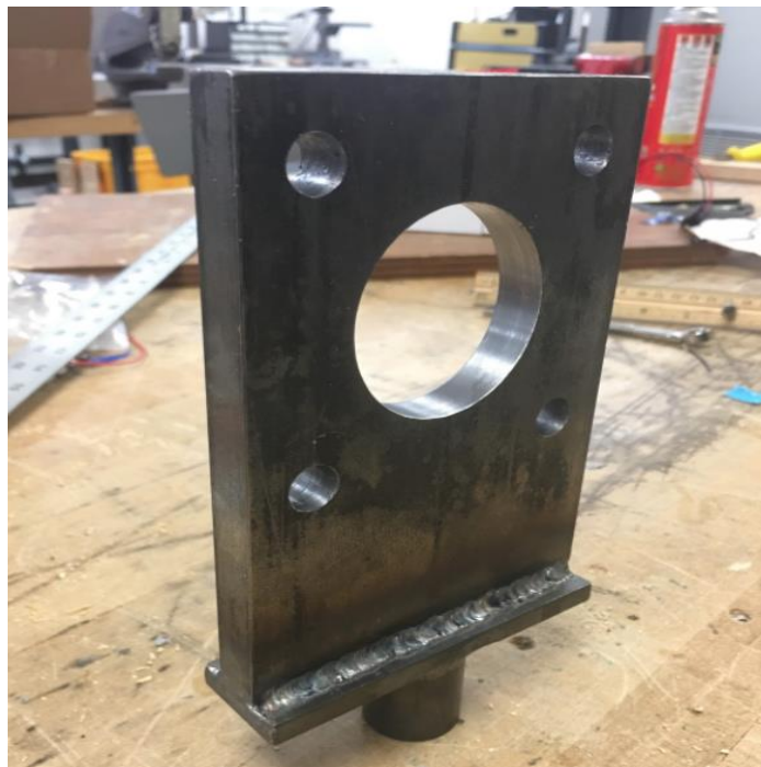
Figure 28 – Bottle jack attachment for front support
