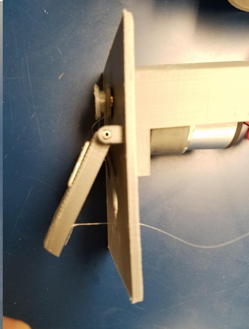
Close up view of ball-and-keyhole style trap door
