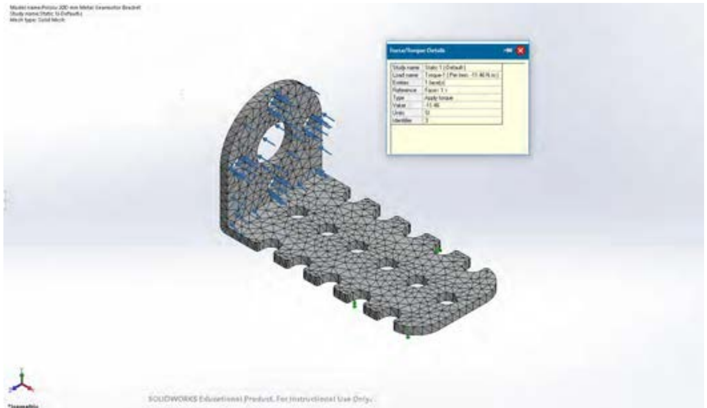
Figure 28: Unloaded model with mesh, loads and boundary conditions
