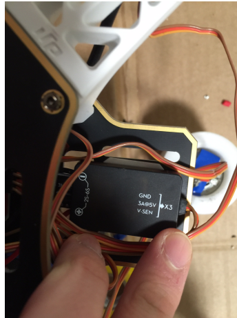
Figures 6.5.2 and 6.5.3: The Naza Lite flight controller and LED module (6.5.2) and its power supply (6.5.3)
