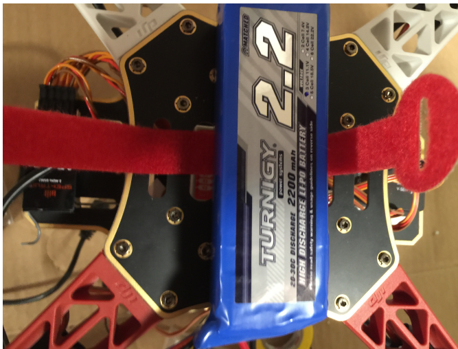
Figure 6.5.6: The 2200 mAh lithium ion battery used to power the drone
