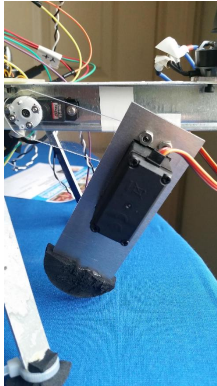
Figure 16: Close up of the hinged landing gear joints
