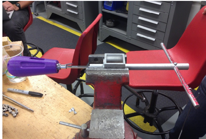
Figure 10: Torque calibration test apparatus.
