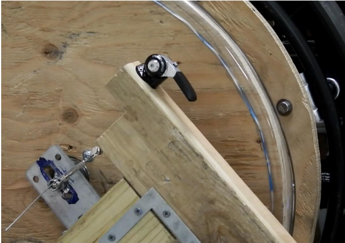
Figure 17 Close-up view of shifting mechanism
