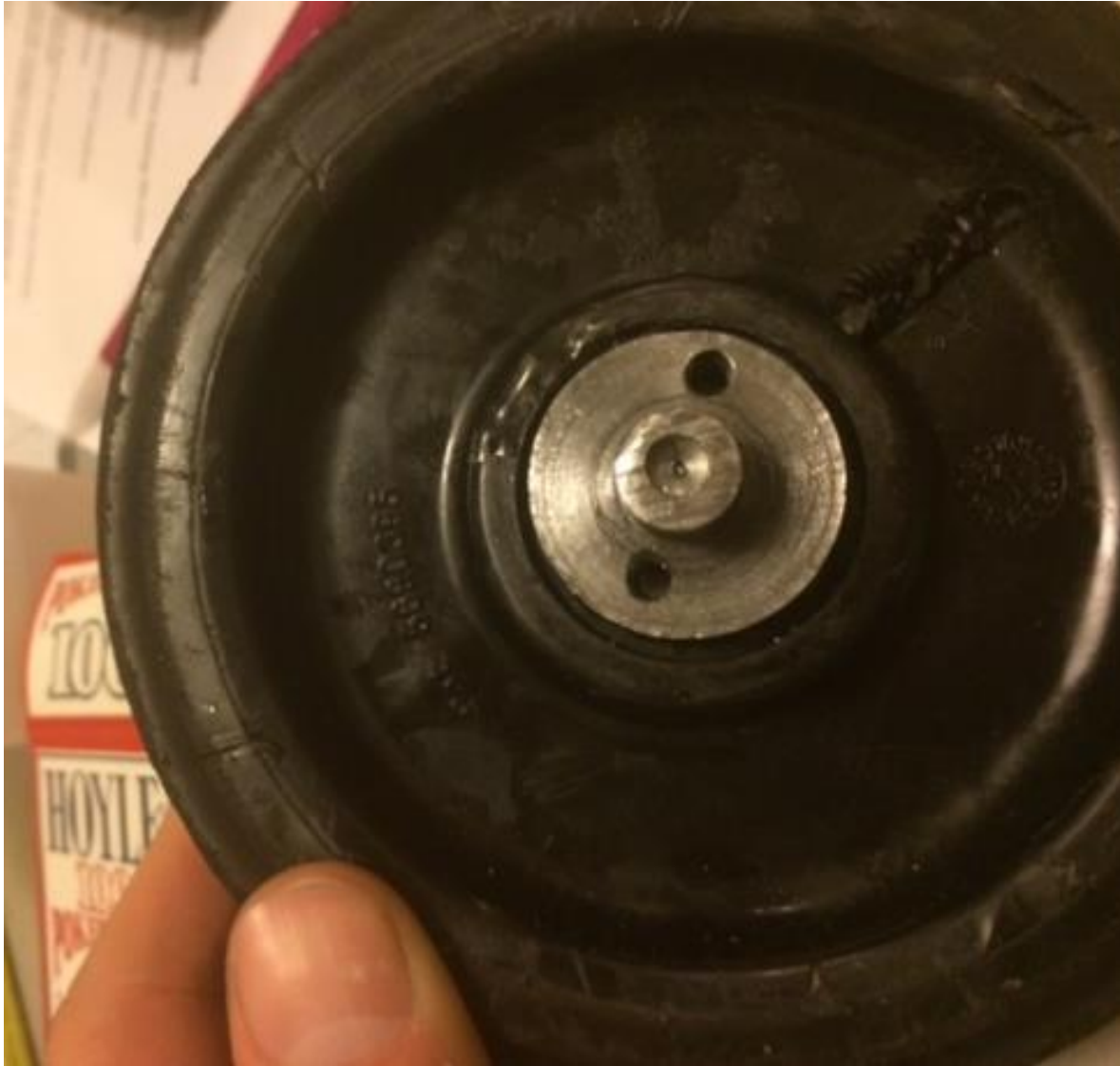
Figure 6.3.6 Stainless steel shaft other side
