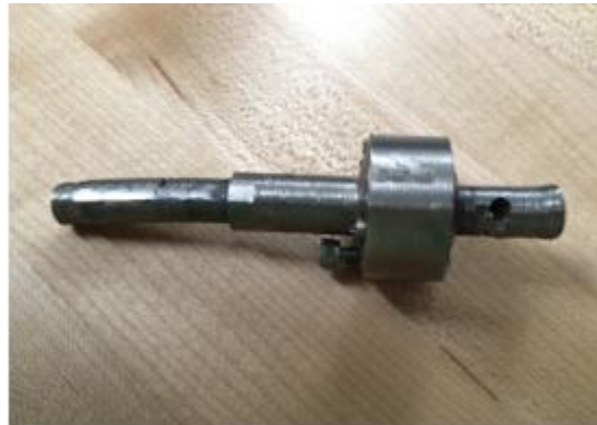
Figure 6.3.3: Warped Aluminum Shaft.
