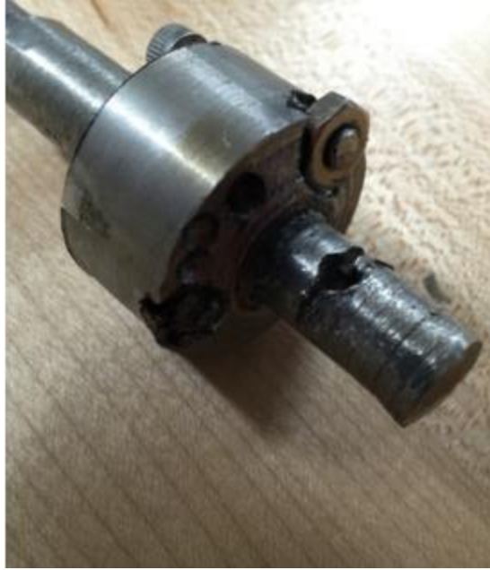
Figure 6.3.4: Aluminum shaft set screw hole
