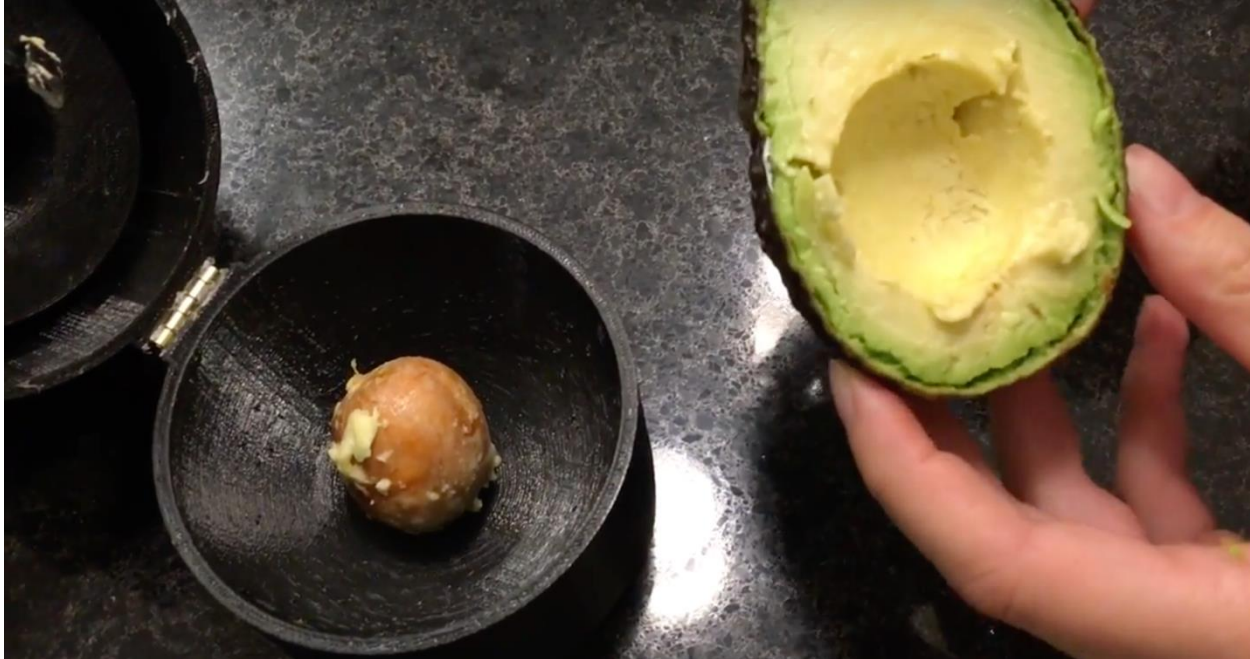
Figure 28 This picture shows an avocado that our pitter extracted the pit from. This image also shows how there was minimal damage to the fruit and minimal fruit left on the pit. This pitter design had been modified to accommodate fruit that was in season: hence the avocado.
