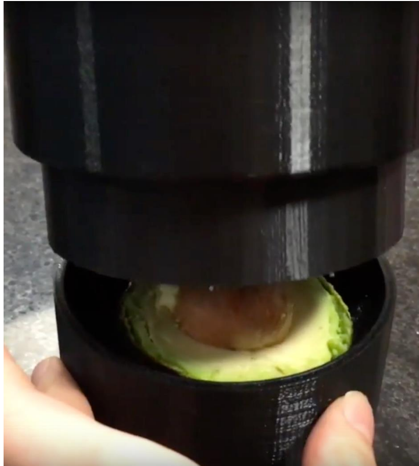
Figure 27 This picture shows how our pitter mechanism is being placed around the avocado pit. The device closes on top of the fruit without damaging it and extracting the pit.
