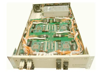
Figure 5.2: Washington University Gigabit Switch Loaded with Four FPX Cards
