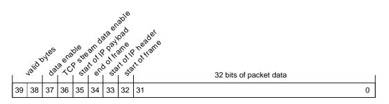
Figure 6.8: Data FIFO data format
