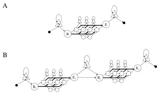
Figure 3.1: (A) The 1-pass HMM structure obtained by eliminating the feedback path from the Plan7 structure. (B) The 2-pass HMM structure obtained by creating two copies of the Plan7 motif separated by a linker state, L, to emit non-motif symbols between them.
