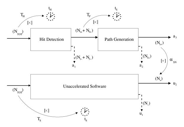
Figure 2.4: The relationship between various quantities introduced in the Performance model of Section 2.2. A straight edge represents a path through the system. Dashed edges represent paths that result in a negative output. The quantity in parentheses next to an edge indicates the number of searches passing through it. An arc represents derivation of the quantity next to it by performing the operation in square brackets on the operands at either end in the direction of the arrow.
