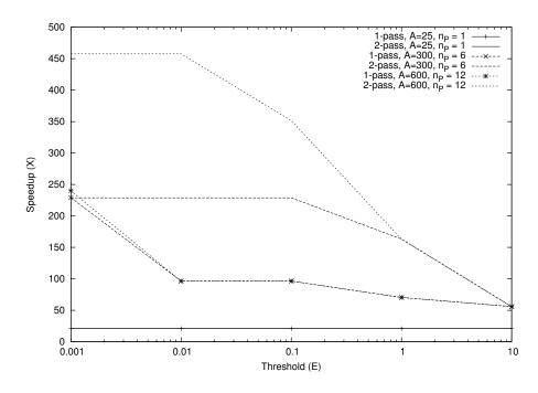
Figure 3.4: An alternative comparison of the speedup achievable by 1-pass and 2pass architectures using estimates for A made on the basis of the published Smith-Waterman performance numbers of Table 3.2. A constant value  $f_{CLK} = 100$ MHz is assumed for all curves in this figure. The plot must be read from right to left in order to consider increasing stringency of threshold E.
