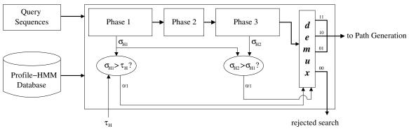
Figure 3.2: The three pipelined phases that make up the Hit Detection stage in a 2-pass architecture. The 2-pass heuristic forwards all searches which see any improvement from  $\sigma_{H1}$  to  $\sigma_{H2}$  to Path Generation, irrespective of whether  $\sigma_{H1}$  exceeds Hit Detection threshold,  $\tau_H$ .
