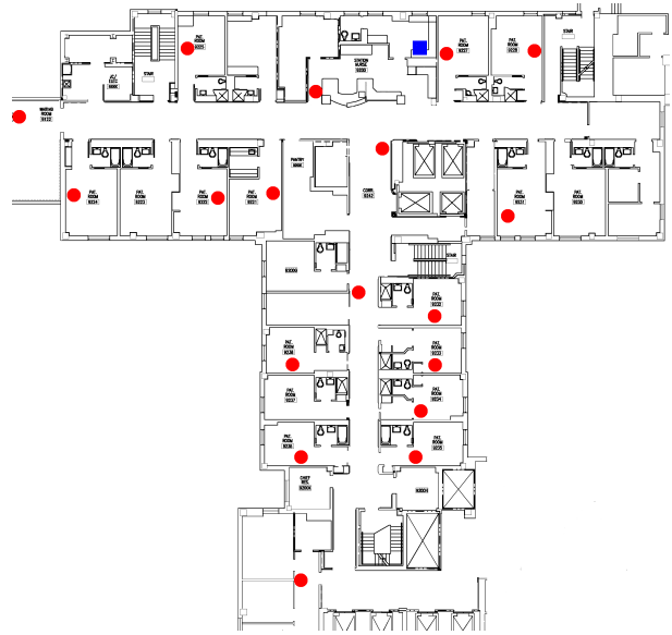
Figure 2: Deployment at Barnes-Jewish Hospitals. The blue square denotes the base station. Red circles denote relay nodes.
