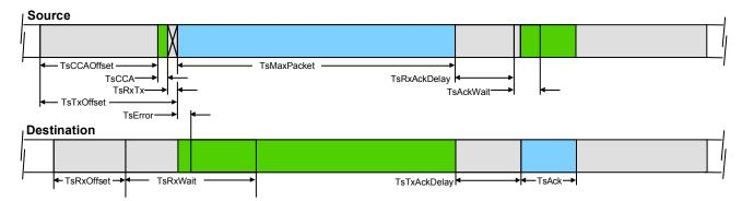
Fig. 2: Transaction timing in one time slot [1]
