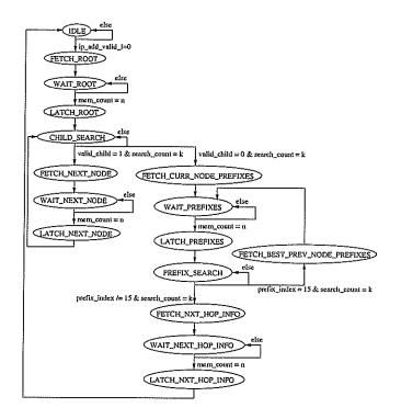
Figure 8: FIPL engine finite-state-machine bubble diagram.
