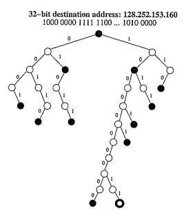
Figure 2: IP lookup table represented as a binary trie. Stored prefixes are denoted by shaded nodes. Next hops are found by traversing the trie.
