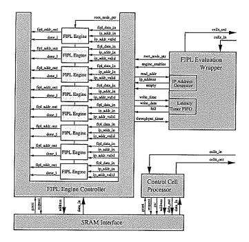
Figure 12: Block diagram of FIPL evaluation environment.
