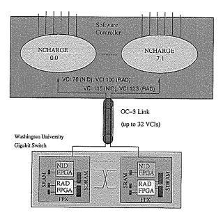
Figure 9: Detail of the hardware and software components that comprise the FPX system. Each FPX is controlled by an NCHARGE software process. The contents of the memories on the FPX modules can be modified by remote processes via the software API to NCHARGE.
