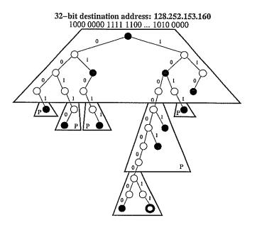
Figure 3: IP lookup table represented as a multibit trie. A stride, 4-bits, of the unicast destination address of the IP packet are compared at once, speeding up the lookup process.
