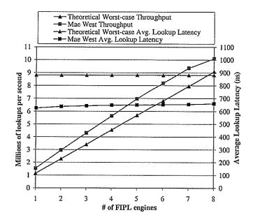
Figure 13: FIPL performance: measurements used a sample database from Mae West on July 12, 2001 consisting of 16,564 routes. Input test vectors consisted of random selections of 2048 IPv4 destination addresses.
