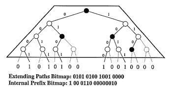
Figure 4: Bitmap coding of a multibit trie node. The internal bitmap represents the stored prefixes in the node while the extending paths bitmap represents the child nodes of the current node.
