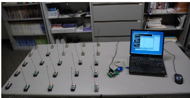
Fig. 8. A 5x5 Mica2 mote test bed
