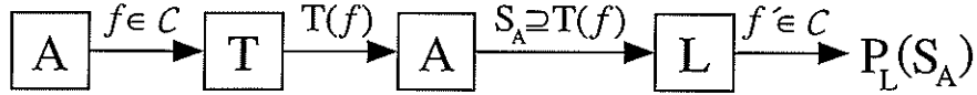
Figure 1: An overview of a teaching session. The adversary chooses the target function, f , giving it to the teacher. The teacher then generates T(f) . Given T(f) the adversary generates S_A \supseteq T(f) and gives this to the learner. The learner (possibly randomized) outputs a representation from \mathcal{C} thus defining a probability distribution P_L(S_A) over \mathcal{C} .
