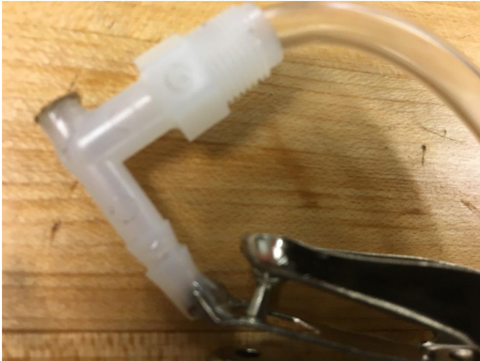
Figure 19: View of Silicon Tubing and Tube Fitting Mounted On Hole Punch
