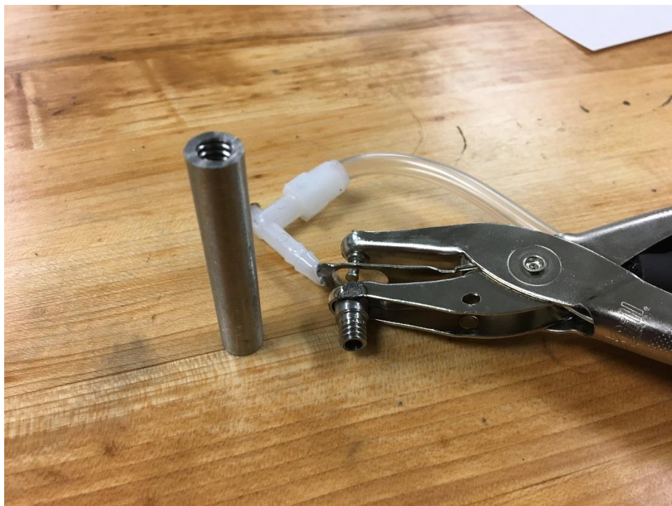
Figure 20: View of The Steel Tube Fitting and Detachable Steel Tube
