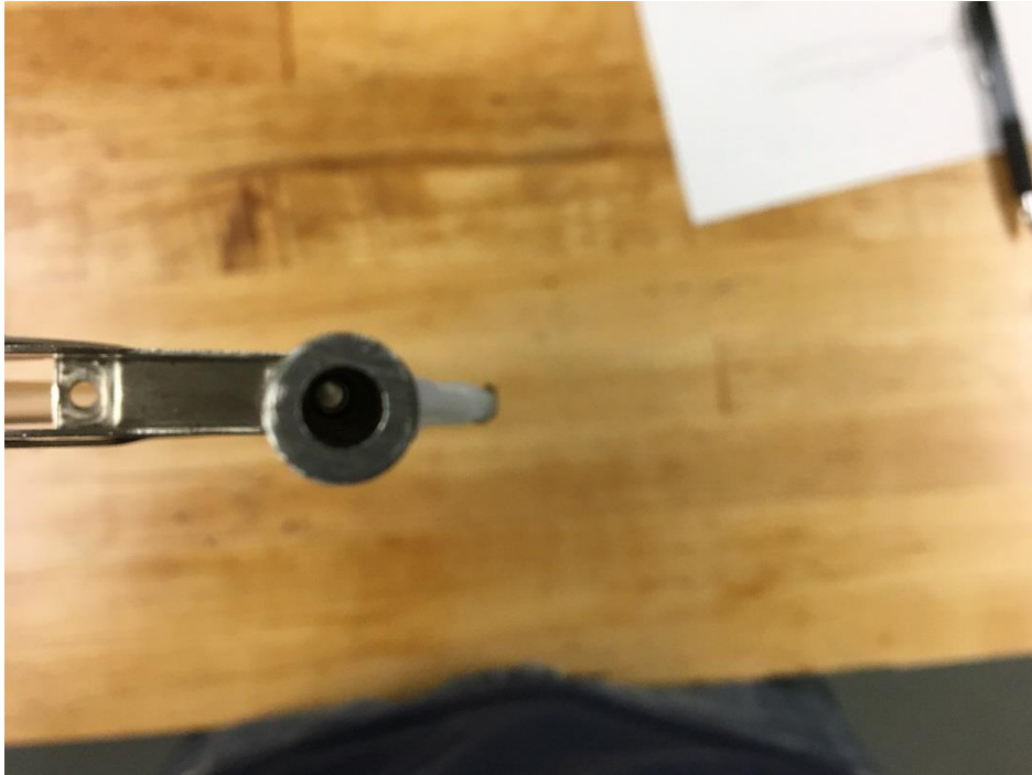
Figure 21: Bottom View of the Tube Showing Hole That Sample Goes Through
