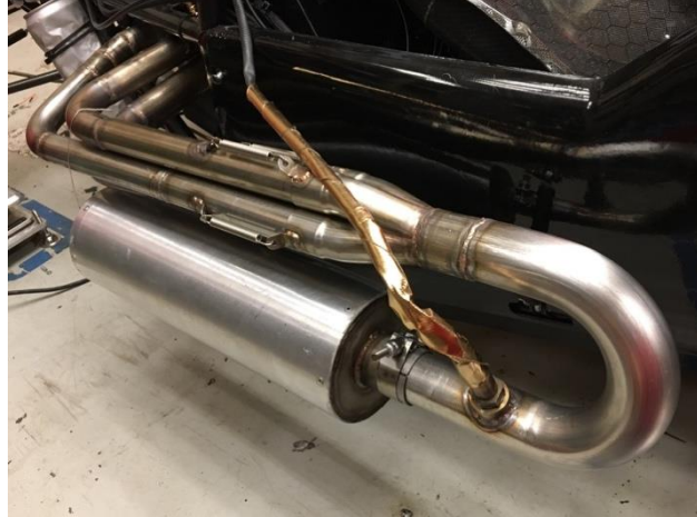
Figure 7. WUFR-19 exhaust system
