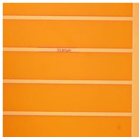
A-3 Dimension of deposited patterns after liftoff
