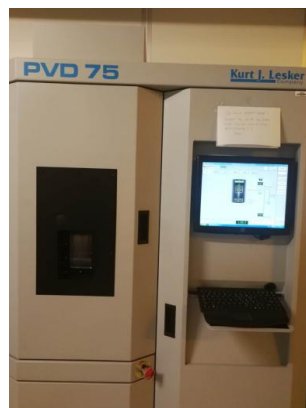
Figure 2.8 Kurt Lesker PVD 75 Physical Vapor Deposition system
