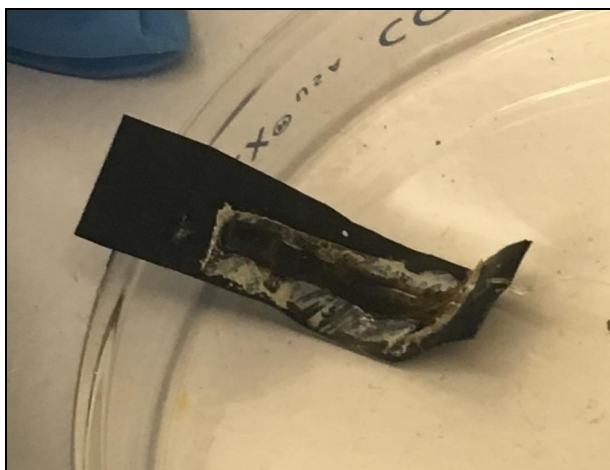
Figure 3.11 Dmaged AMM after 5 hours of irradiation.
