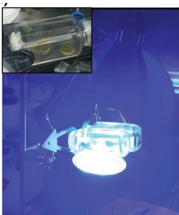
Fig. 3.3 Experimental setup for blue-light irradiation.
