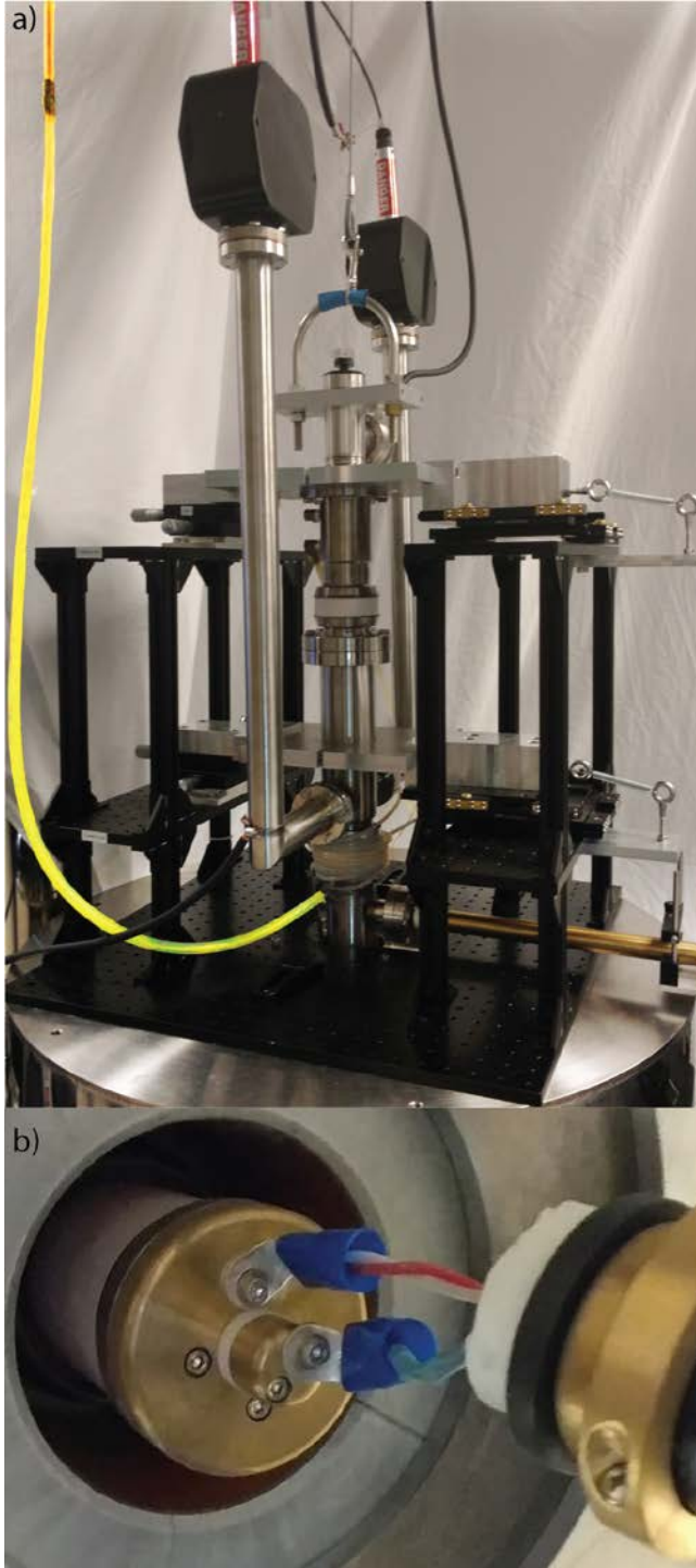
Figure 2.2 a) Photograph of the gyrotron in the magnet. The anode is connected to the low capacitance amplifier by cord highlighted in yellow. Black alignment stages are mounted to the top of the magnet. b) Cathode connection to high-voltage power supply.
