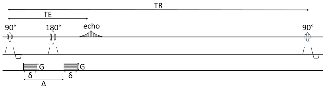
Figure 2.1 Schematic of a typical pulse sequence used in to acquire diffusion data. 90° RF pulse excitation flips the protons perpendicular to applied magnetic field ( B_0 ). The protons precess about B_0 at varying frequencies, with the precession occurring along the transverse (T2) and longitudinal axes (T1) of the spins. Application of a gradient short after the excitation pulse adds to the phase of each spin. Following the refocusing 180° RF pulse, a second gradient pulse is applied, designed to reverse any phase shifts that occurred due to the first pulse. Water molecules that have moved during the time between the two gradient pulses will not experience a reversal in phase shifts, resulting in a signal decay caused by diffusion. Application of crusher gradients is meant to eliminate any extraneous free induction decay signals if the refocusing RF pulse does not completely reverse phase shifts induced by the excitation pulse.
