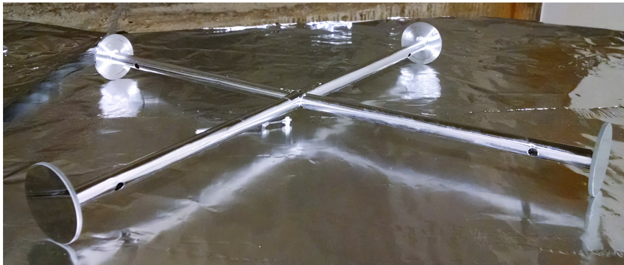
Figure 4.2: The balance before installation. The mirrored \text{SiO}_2 masses are in the foreground.
