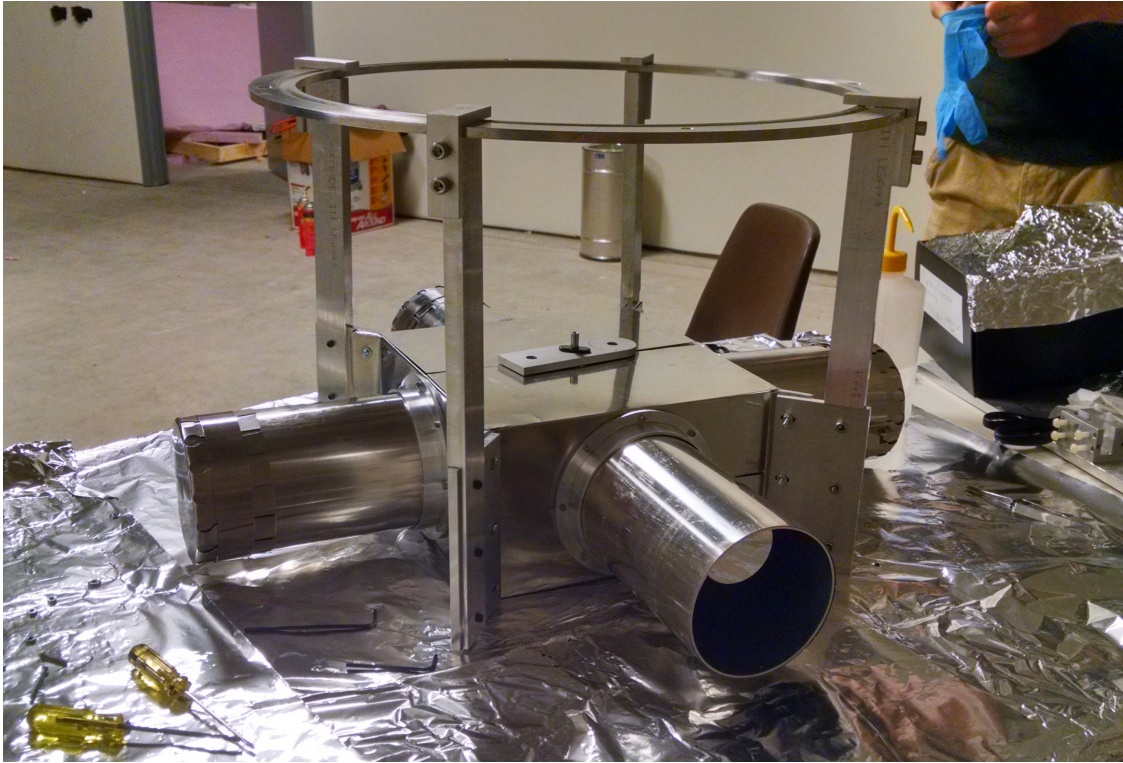
Figure 4.8: The mu-metal magnetic shielding and support structure. The mirrored \text{SiO}_2 test mass used to monitor the position of the balance can be seen in the open end of the shielding tube.
