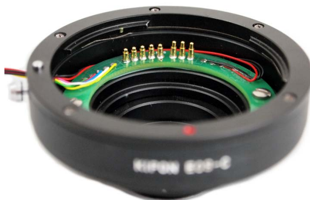
Figure 5.3 The customized Canon EF-S to c-mount lens adapter with spring-loaded pins for electronically controlling the lens.
