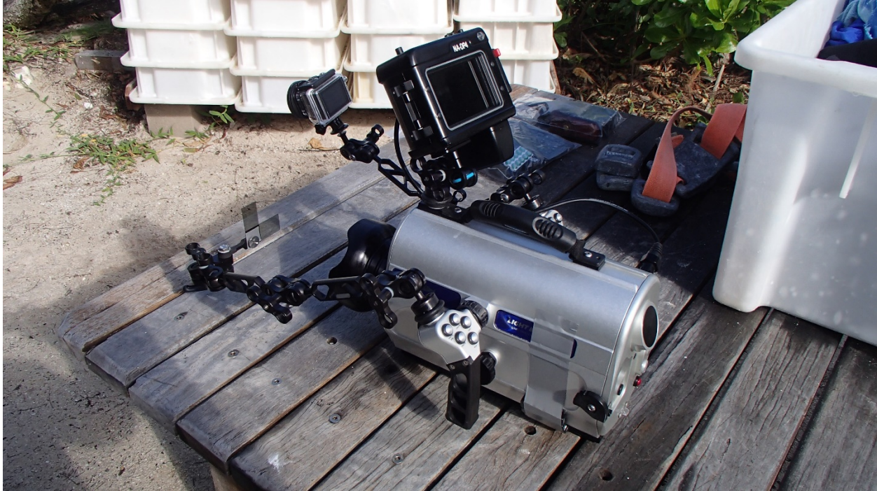
Figure 5.6 The camera, sealed and prepared for a dive. The monitor is mounted on the top of the housing. A small color video camera is mounted on an arm to the right of the housing, and polarization filters are on the left. Extra ballast is taped to the rear of the housing to balance the weight of the monitor.
