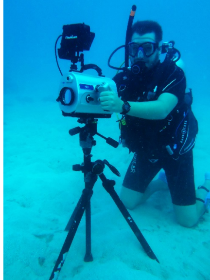
Figure 6.10 The underwater polarization camera prepared for a sun position inference experiment.
