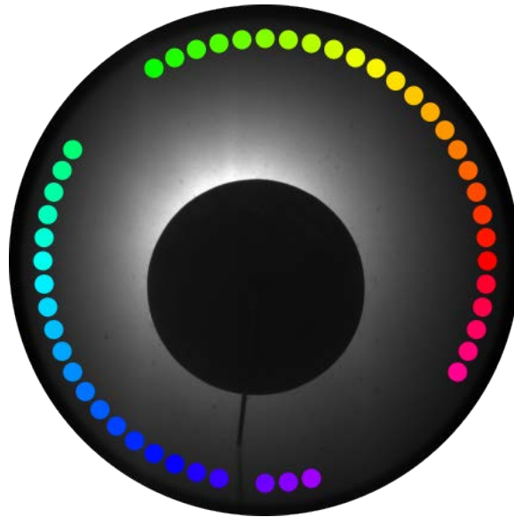
Figure 6.15 An intensity image taken during the sensitivity experiment. The black disk in the center is to block the sun from over-exposing the image. The colored dots around the periphery show the sampling locations for the analysis. Sampling locations were rejected if the DoLP drops below 5% at any point during the analysis.
