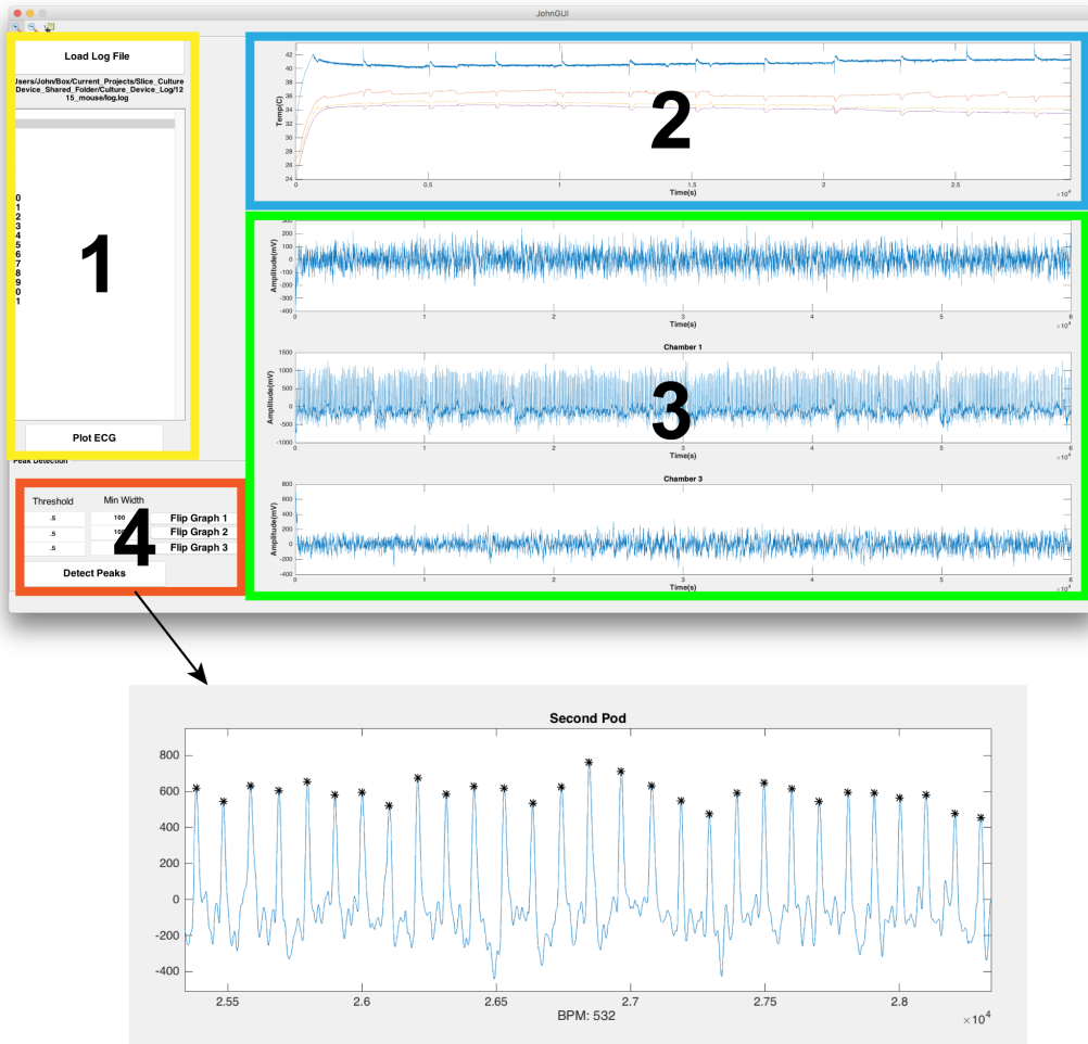
Figure 4.5 Custom monitoring and analysis software. The main graphical user interface consists of 4 sections. Section 1 is for loading the device log and for selecting ECG recordings. Section 2 shows a history of the device temperature. Section 3 shows the pseudo ECG recorded from the culture chambers. Section 4 is used for performing heart rate calculation with user selectable peak detection parameters.
