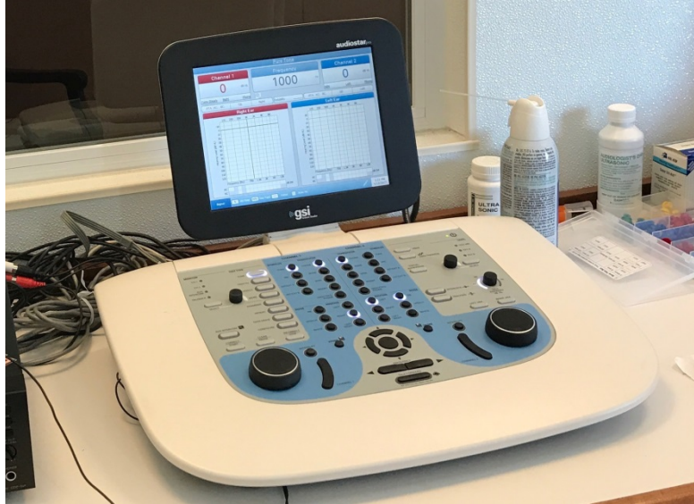
Figure 1.1: A standard clinical audiometer. This device allows for manual delivery of highly-calibrated pure tones at standard audiological frequencies and a variety of sound levels.
